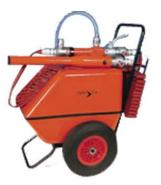
The Delta DF130 Mobile Foam Unit, ideal for protecting oil storage and other high risk areas, is ergonomically designed for rapid one man deployment. The unit requires a connection to a suitable pressurized water supply. Filled with 3% foam concentrate the DF130 will give a running time of approx. 20 minutes, with a foam output of over 34,000 litres of finished low expansion foam.
